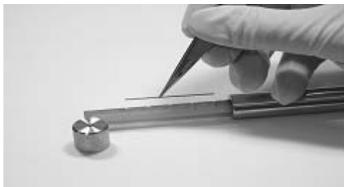
Figure 6: Removing RAPID Strand from spacing jig
